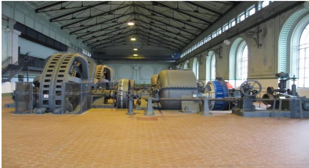
The Bertini plant of 11.000 GWh per year was commenced in 1898. The original Francis hydro turbine is on the right and generator on the left.
