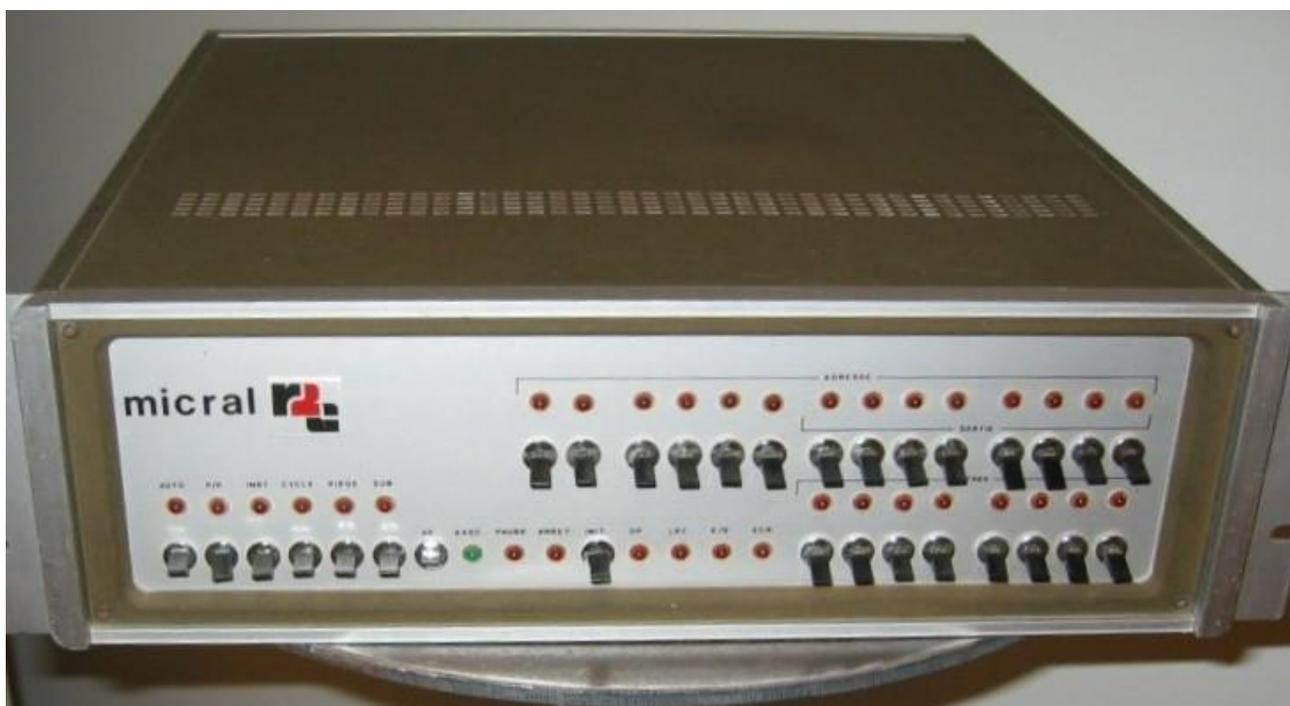
Engineered by the French [François Gernelle](#) for the company R2E (*Réalisations d' Études Électroniques*), the Micral N was the first micro-computer (micro-ordinateur) in the world based on the [Intel 8008 microprocessor](#).
