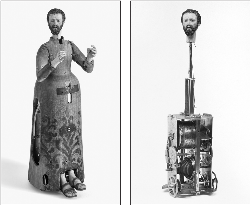
Figure 1. “Preaching Monk” Automaton, ca. 1560, Manufacturer: unknown. This early automaton figure is fully mechanical and performs various repetitive movements. The monk moves on wheels, while its feet imitate walking, and its arms and head move too. Of particular note are the eye and mouth movements, which are controlled by a delicate, precise mechanism in the figure’s head and are particularly remarkable for the time period. (Photo: Deutsches Museum.)
