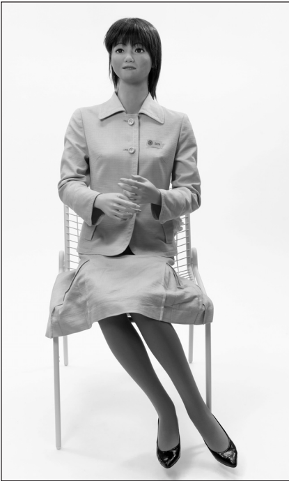
Figure 3. Saya Humanoid Robot, Hiroshi Kobayashi, University of Tokyo, 2009. Saya is a humanoid robot that was designed to be used as a receptionist, a secretary or even a teacher. (Photo: Deutsches Museum.)
